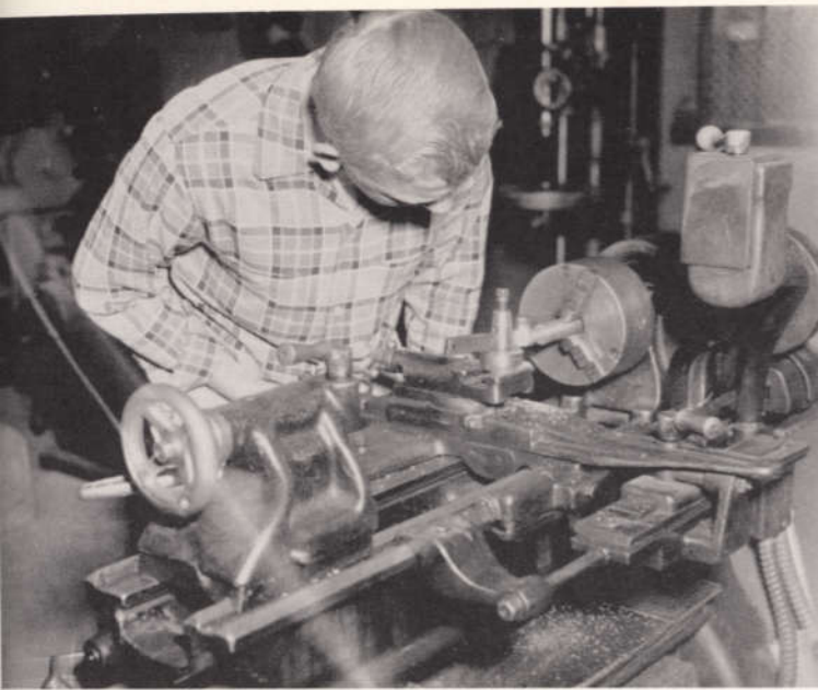
Above, Douglas Bye faces round stock on a metal lathe, an additional piece of new equipment to the Industrial Arts Department.
