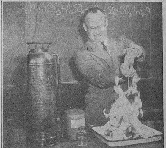
Mr. Orville E. Torgerson puts out the fire he has just set for purposes of demonstration. He is using a miniature fire extinguisher which contains the same type of baking soda and sulfuric acid solution as does the regular extinguisher at his side.
